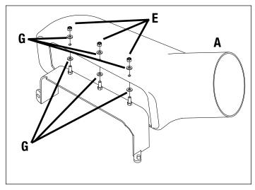
**NOTE:** The deck boot bracket is designed to mount the deck boot on an angle for improved material flow and increased clearance during operation.
