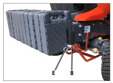
2b. For Lonestar/Deere suitcase weights, slide the Retention Rod (B) through both holes on the top of the Weight Bracket and insert Hairpin Cotters (E) in the two center holes on the Retention Rod.
