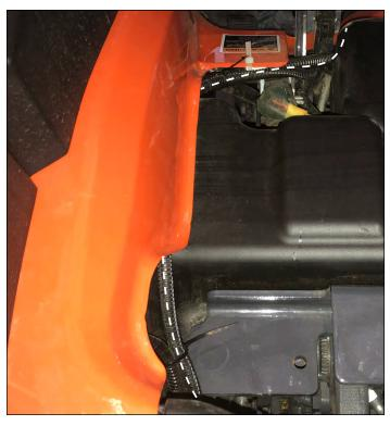
The harness then follows the tractor's existing wires across the rear of the tractor and up the ROPS on the right side.
