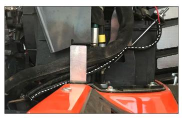
3. Under the tractor, follow wiring toward the rear of the tractor and thread it up through the opening located at the front left side of the tractor seat.
