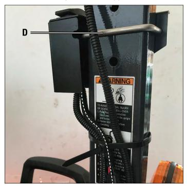
7. Use the Zip Ties (F) to secure the Wiring Harness to the tractor's existing wiring. Apply these to areas to prevent wires from hanging too low and/or making contact with moving parts.
