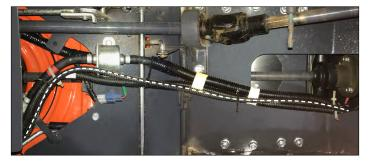
Lift the seat. Route the Wiring Harness alongside the existing wiring towards the rear of the seat and then back under the rear fender.
