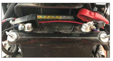
Open the tractor's hood. The Wiring Harness should follow the existing wires forward, down through the opening at the left side covered by the rearmost portion of the hood.
