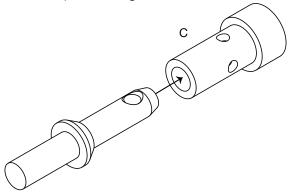
3. Using a hammer, tap the roll pins (D) through the holes.
