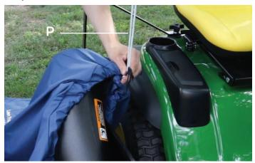
10. Attach the S-hook (Q) through the metal grommet on the Leaf Bag.
