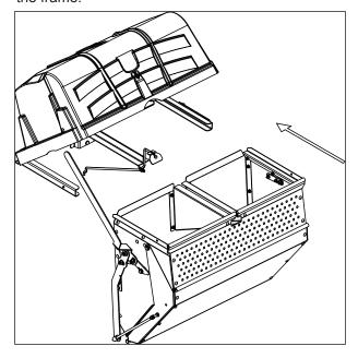
2. Use 1/4" x 3/4" clevis pin (A) and bowtie clip (B) to secure bin on left side.
