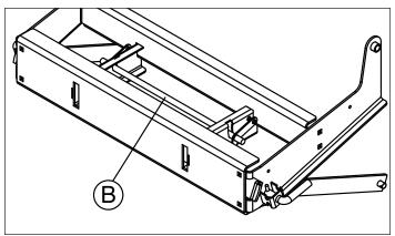
To release an attachment, lift rod (B) and slide the attachment forward slightly. This will unlock it, enabling it to be pulled out.
