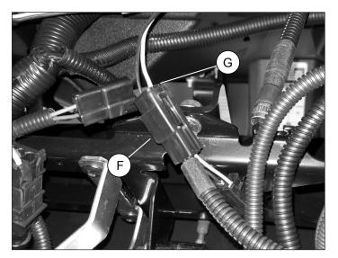
9. Route the circular connector down towards the bottom of the underside of the dash
