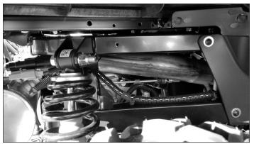
Position the two connectors (T) at the end of the power harness 2 – 3 inches beyond the end of the frame rail and use a wire tie to secure the harness to the upper holes (U) of the vertical shock mount.
