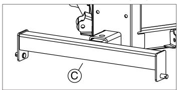
Attach frame assembly (D) to mounting brackets using two 1/2" x 1-1/2" clevis pins (E). Fasten clevis pins with bowtie clips. It is recommended that two people do this installation.
