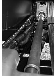
6. Insert the circular connector of the power harness through the hole (E) in between the plastic panel and the frame rail and push it up into the upper area of the dash below the cup holders
