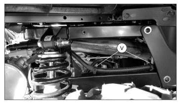
21. Working back toward the battery compartment, secure the harness to the main chassis harness with wire ties at least every 10" and on both ends of a bend. If necessary, coil up and secure any excess length of harness near the accessory port.
