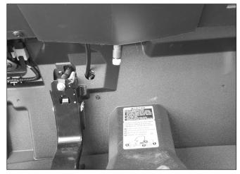
10. Attach the display cable (H) to the display (J).
