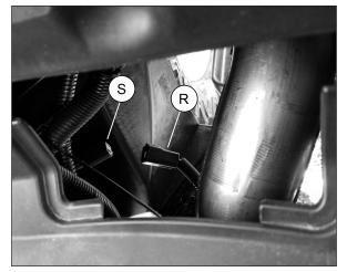
18. Route the power harness toward the rear of the vehicle along the top side of the lower frame rail.
