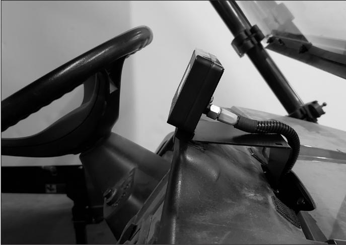
7. Route the display cable (S) to the right of the hood latch and connect to the power harness (T).
