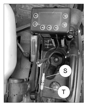
13. Connect the battery harness to the battery. The black harness wire connects to the negative battery terminal and the red harness wire connects to the positive battery terminal. The wires should exit the battery terminals toward the center of the battery.
