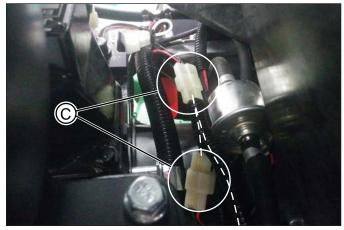
7. Continue routing the power harness under the operator station platform to the ROPS at the right rear of the tractor by following the main chassis harness. Secure the power harness to the main chassis harness at least every 10" and on both ends of a bend
