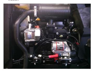
Locate and disconnect the fuel pump connector (B).
