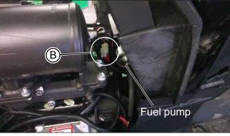
6. Plug the wire harness pigtail (C) in-line with the fuel pump connectors.
