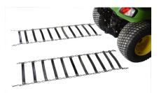
1) Lay the tire chains out on the floor behind or in front of the rear tires of the vehicle, with the peened side of the rivets up (head down). The hook goes to the inside and the latch to the outside of the tire.
