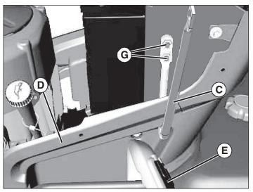
2. Install end of lever bracket (C) through an existing hole in the removable console panel (D), inside the lift pedal (E), at the left side of the machine.
