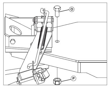
Install 1/2 x 1 in. bolt (O) through hole and secure with 1/2 in. locknut (P).
