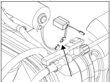
Expose adhesive backing located on the back of the remote receiver box and adhere the receiver box (A) close to the electric motor but out of the way of hoses, cap or moving parts.
