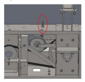
1.)Note the length of exposed threads on tension rod and loosen nut to remove tension from drive belt on blower
