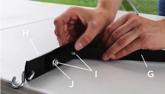
5. Secure the Bag Bracket in place using the two 1/4 in. Flange Nuts (J). The angled section at the end of the attached Guide Bracket should be facing away from the tractor.
