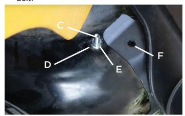
3. Slip the rear hole (F) in the chute over the bolt installed in step 2.
