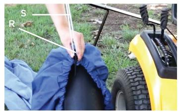
8. Hang Leaf Bag on S-hook (T) using Grommet. To prevent interference and tangling, hook the drawstring (U) onto the S-hook.
