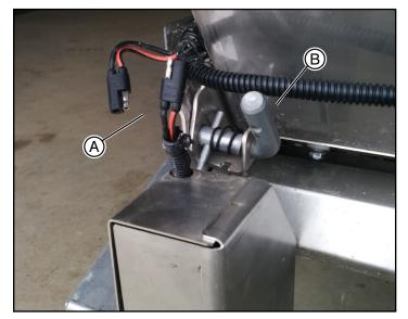
Lock out the pins (B) on both sides of the machine. When the second pin is pulled, the rear of the tray will drop.
