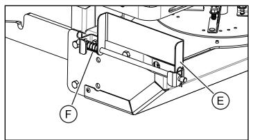
The barrier shield (E) comes installed on the left side of the fertilizer spreader. To raise or lower the shield, push it against the spring (F) and rotate.
