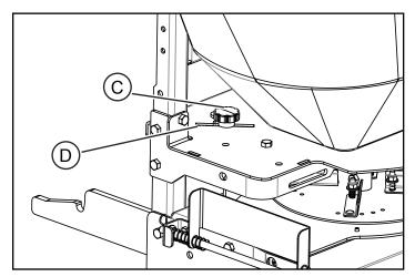
2. Position the knob in the end of the slot at position (D) for maximum material output.
