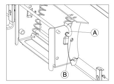
To prevent damage to blade extensions, be sure the blade trip lock pin (A) is not engaged in hole (B). If pin is in hole, pull out to disengage and turn vertically into slot.
