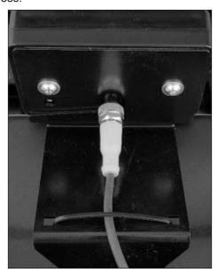
12. Mount the display by sliding the bracket into the receiver. Press down on the bracket firmly.
