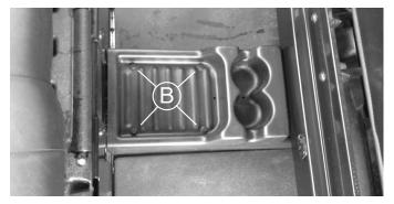
2 seat Gator - Lift the passenger seat to access the battery. Route the end of the harness with the circular connector from the battery compartment down into the center channel to the front of the vehicle behind the dashboard following the vehicle wiring harness.
