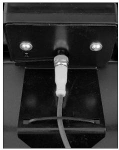
12. Mount the display by sliding the bracket into the receiver. Press down on the bracket firmly.
