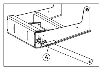
If you wish to raise the bed without removing the attachment mounting frame, it can be folded down by pulling the Pins (A) and turning to lock them out. (Lift up on the frame when pulling the second pin and lower gently to the ground). To put the attachment mounting frame back into position, release the pins and lift the frame until it clicks into position.
