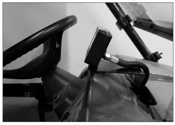
13. Route the display cable (S) to the right of the hood latch and connect to the power harness (T).
