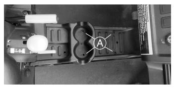
4 seat Gator - Remove four additional plastic pins (B) to remove the rear center cover. Remove the front seat and plastic storage compartment to improve access to the center channel.
