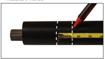
4. Using the cut off portion of the guard mark (B) and cut that distance from the driveline tube.
