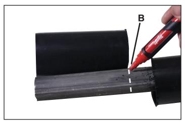
Note: The driveline tube should protrude approx. 1.25 - 1.5 in. past the guard.
