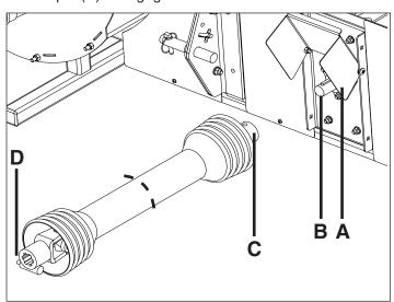
3. Lift the tractor's 3-point arms up and down to ensure that the PTO telescopes freely, does not come apart and does not bind.
