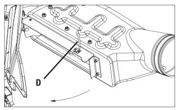
4. With boot against mower deck, lower handle (E) rearward to secure boot (shown with no dicharge chute for clarity).
