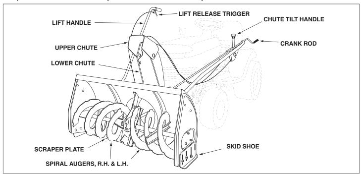
**CHUTE TILT HANDLE** Pivots the Upper Chute up or down to control the angle and distance of discharge. **CRANK ROD** Rotates the Lower and Upper Chutes to control the direction of discharge.
