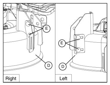
Connect brush support assembly to mower mount brackets at desired height (see page 4) using 3/8" x 3-1/2" Carriage Bolt (G), two Spacers (H), 3/8" Flat Washer (J), 3/8" Star Washer (K) and 3/8" Lock Knob (L). Thread 3/8" Lock Nut (M) onto the ends of the threads to prevent lock knobs from vibrating off.
