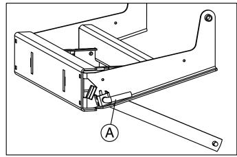
If you wish to raise the bed without removing the attachment mounting frame, it can be folded down by pulling the Pins (A) and turning to lock them out. (Lift up on the frame when pulling the second pin and lower gently to the ground). To put the attachment mounting frame back into position, release the pins and lift the frame until it clicks into position.
