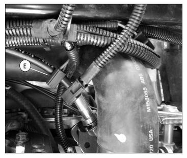
Loop the remainder of the harness under the frame rail and attach to the outside of the right frame rail. Allow the 2 connectors to extend 2-4 inches past the end of the frame rail and secure with a wire tie trough hole (F). Secure the harness to the frame rail with clips (G).
