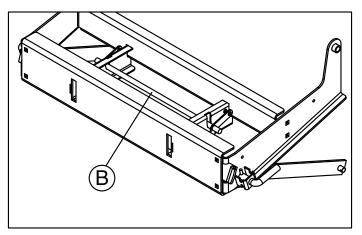
To release an attachment, lift rod (B) and slide the attachment forward slightly. This will unlock it, enabling it to be pulled out.
