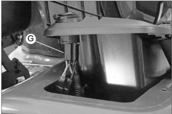
7. Reinstall the toolbox and tighten the M10 nuts on toolbox and the M13 nuts on the handle. Route the two connectors on the free end of the power harness through the elliptical hole in the frame (H) and secure with a wire tie through a nearby hole. Remove any slack in the harness by pulling on the circular connector in the toolbox.
