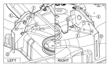
Connect brush support assembly to mower mount brackets at desired height (see page 4) using 3/8" x 3-1/2" Carriage Bolt (J), two Spacers (K), 3/8" Flat Washer (L), 3/8" Star Washer (M) and 3/8" Lock Knob (N). Thread 3/8" Lock Nut (P) onto the ends of the threads to prevent lock knobs from vibrating off.
