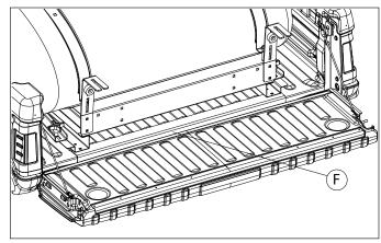
2. Lower tailgate, center sprayer in utility vehicle bed with rear channel lip (F) inserted between bed and tailgate. Be sure lip is tight against bed.
