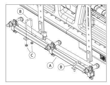
1. Install boom (A) as shown using two u-bolts (B) and four 5/16" flange nuts (C).
