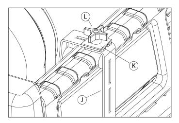
5. Position the outer boom support (J) below the inner boom support with the square plate (K) on top. Push it as far into the slot as possible and tighten the lock knob (L).
