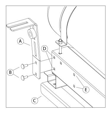
NOTE: Use outer holes (D) for 150" boom and inner holes (E) for standard utility vehicle boom and boomless.
