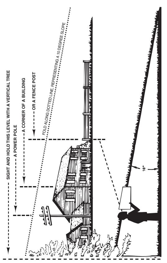
CAUTION: DO NOT OPERATEYOURTRACTOR AND CART ON A SLOPE IN EXCESS OF 10 DEGREES. BE SURE OF YOURTRACTOR'S TOWING AND BRAKING CAPABILITIES BEFORE OPERATING ON A SLOPE.
